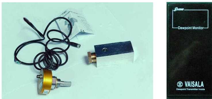
Picture 6-6: Parts of Dew-point Monitor
