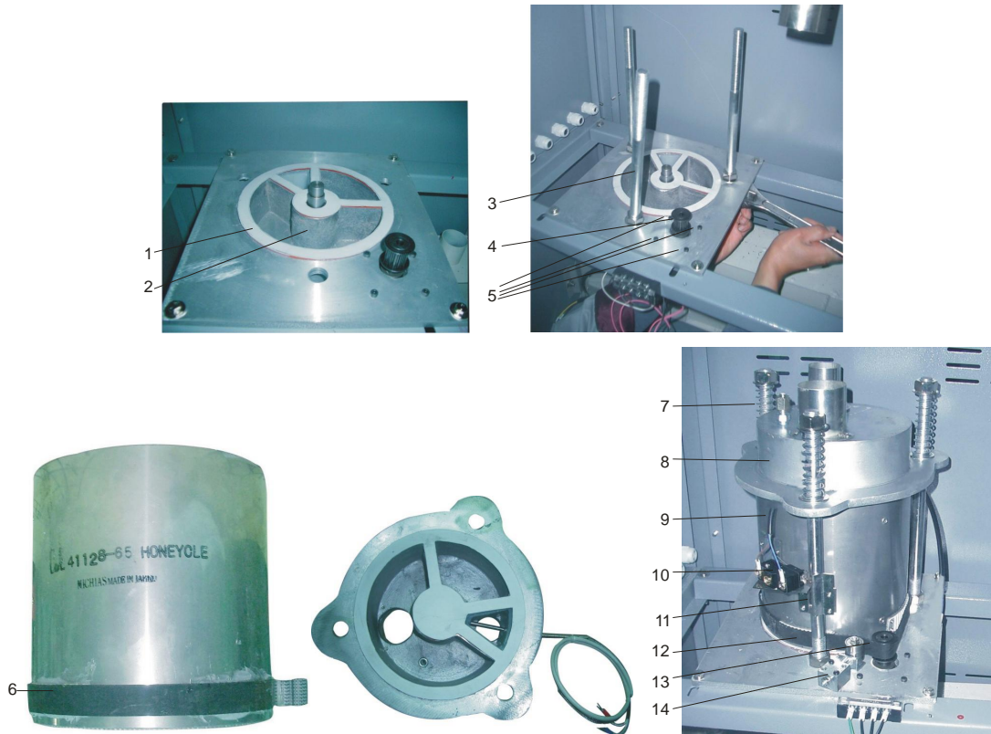
Picture 6-3: Installation of The Rotor
