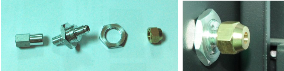
Picture 6-7: Copper Joint Assembly of Original Machine
