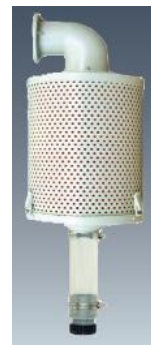
Picture 3-4: Left: Air-exhaust elbow of dryer Right: Air-exhaust filter
