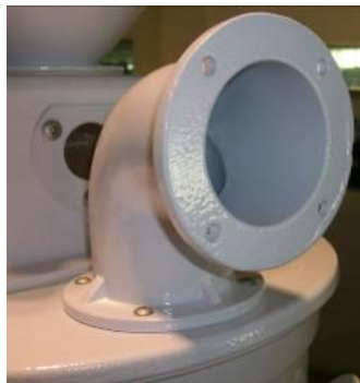
Picture 3-4: Left: Air-exhaust elbow of dryer Right: Air-exhaust filter
