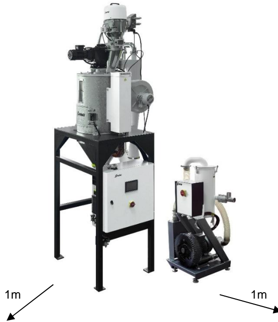
Picture 3-2: Machine Installation Distance
