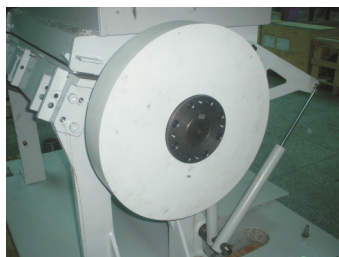
Picture 6-13: Installation of Belt Pulley and Motor 4 (SG-3675)
