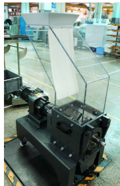
Picture 6-9: Installation of Feed Box, Feed Port and Storage Bin 2
