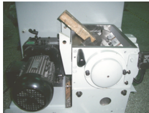
Picture 6-2: Dismantle Fixed Blades
