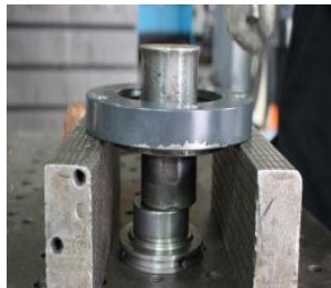
Picture 6-16: Step 1 of Bearing Dismantlement
