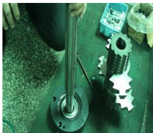
Picture 6-15: Step 3 of Left/ Right Bearing Base Dismantlement
