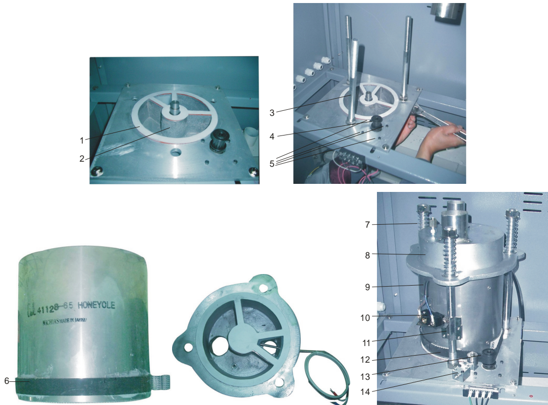
Picture 6-3: Installation of The Rotor
