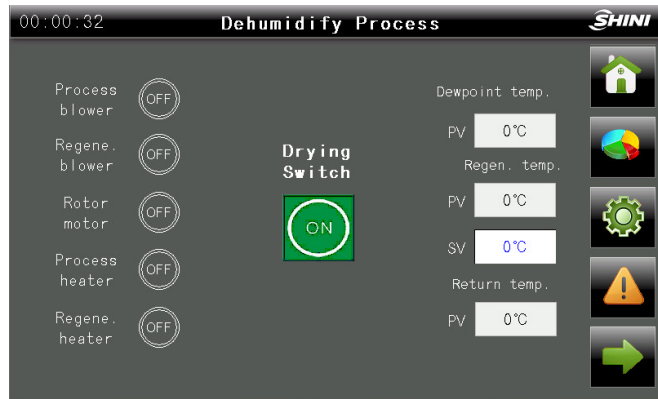
Picture 4-15: Dehumidify Process Screen
