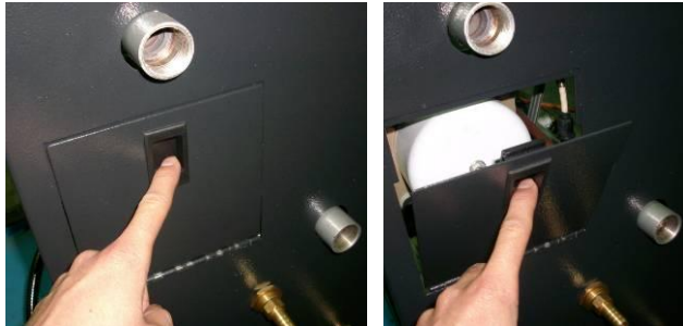
Picture 6-6: Pipe Heater 1
