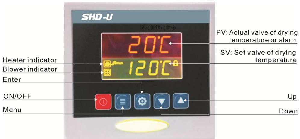
Picture 4-1: Control Panel
