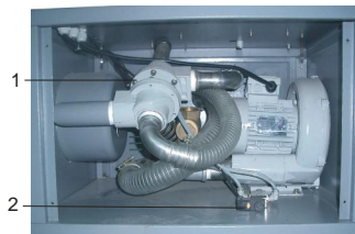
Picture 6-4: Conveying blower
