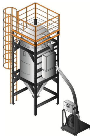
Picture 2-3: Safety Ladder
