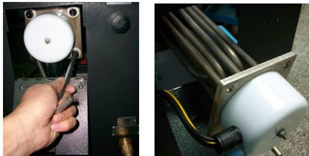
Picture 6-4: Heater Pipe 2
