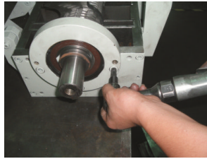
Picture 3-9: Installation of Rotating Blade and Fixed Blade 2
