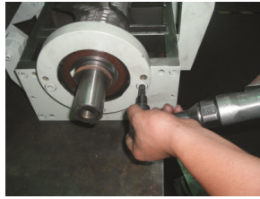
Picture 3-5: Installation of Bearing and Blade Rest 3
