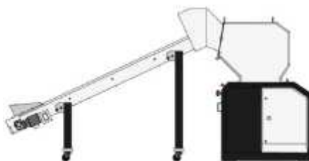
Picture 6-2: Feeding Hopper for Conveyor
