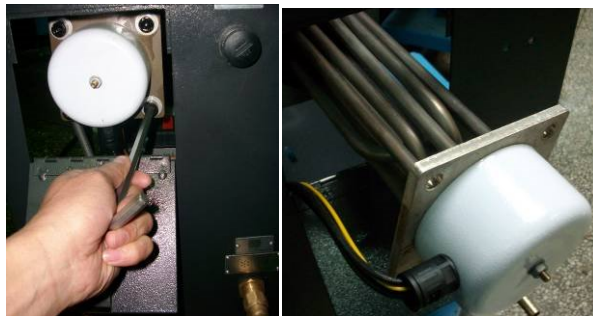
Picture 6-7: Pipe Heater 2
