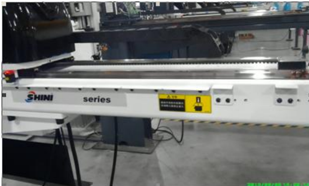
Picture 3-3: Outside IMM safety zone blocks before modified
