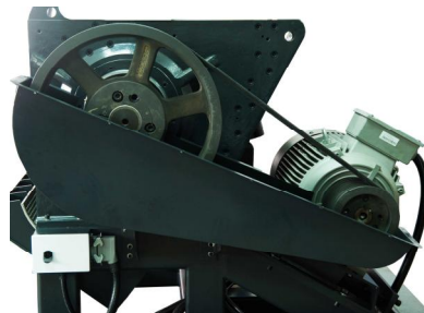
Picture 6-6: Installation of Belt Pulley and Motor 2
