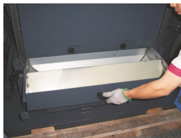
Picture 6-13: Installation of Storage Box, Screen and Screen Bracket 5
