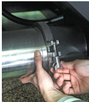
Picture 4-3: Loosen the Fast Pipe Clamp
