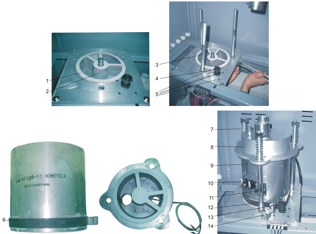
Picture 6-3: Installation of The Rotor
