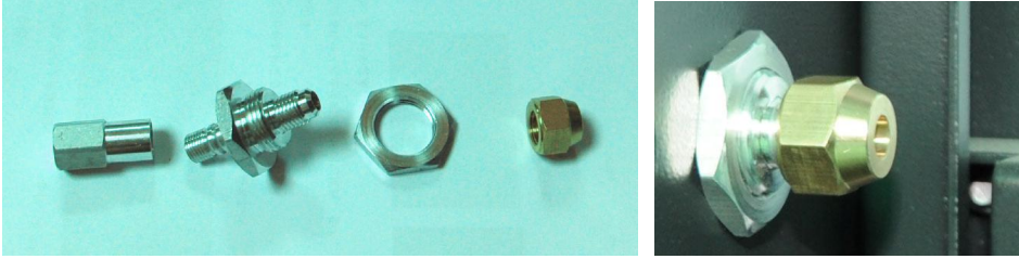
Picture 6-7: Copper Joint Assembly of Original Machine
