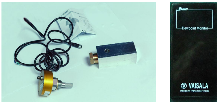
Picture 6-6: Parts of Dew-point Monitor
