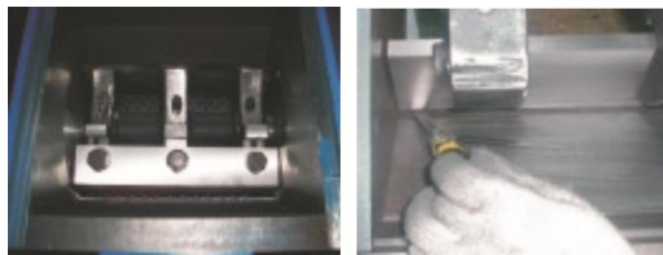
Picture 3-3: Installation of Rotary Blade and Static Blade
