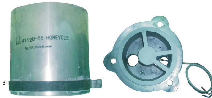
Picture 6-4: Honeycomb-rotor installation steps 3
