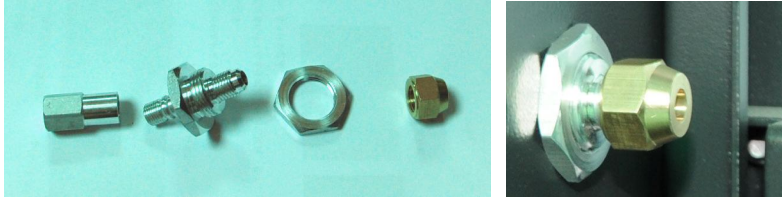
Picture 2-13: Copper Joint Assembly of Original Machine
