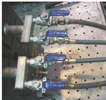
Picture 3-3: Mould and Water Coupling 2
