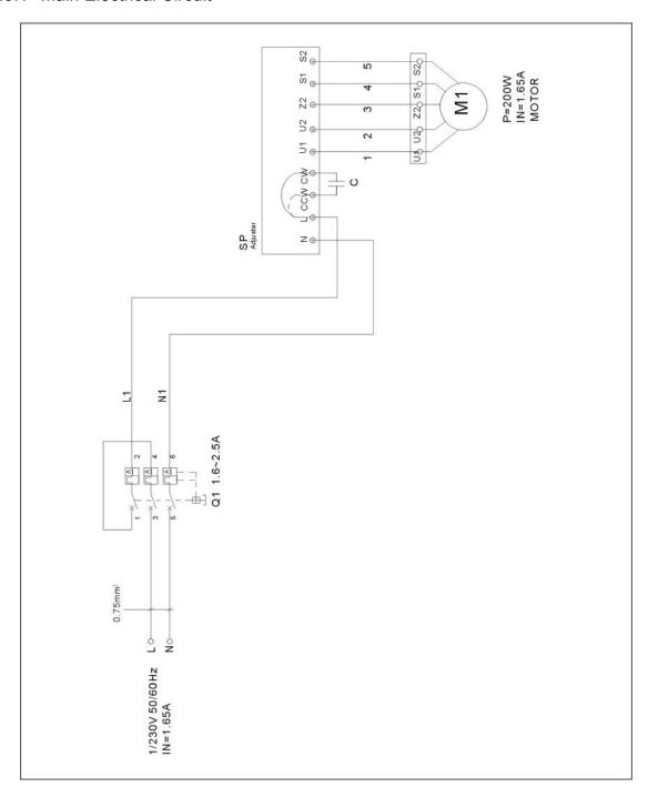
Picture 2-2: Main Electrical Circuit
