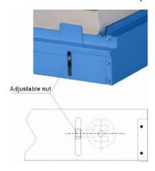
Picture 4-3: PVC Belt Adjusting Drawing
