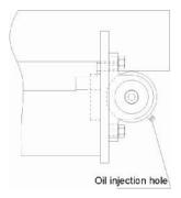
Picture 6-2: Bearing Lubricate Drawing
