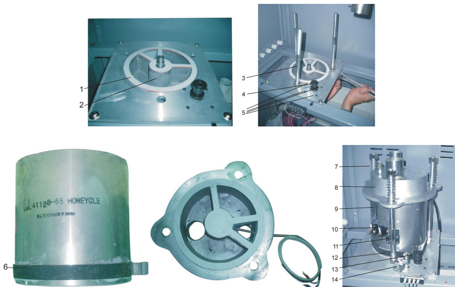
Picture 6-3: Installation of The Rotor (SD-40H~700H)
