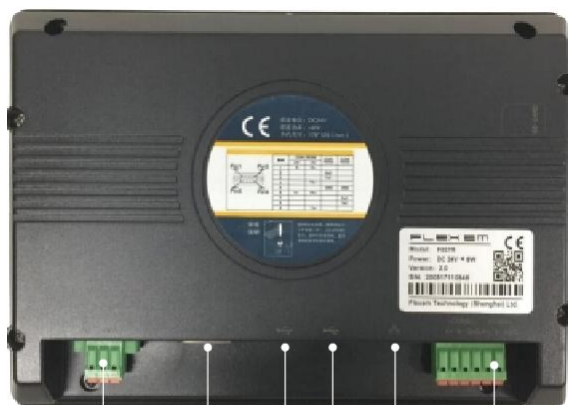
Power terminal DB9 serial port USB Host USB Slave Ethernet port 485 terminal
