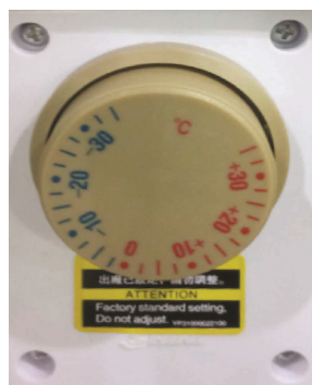
Picture 3-14: Compressor anti-freeze switch
