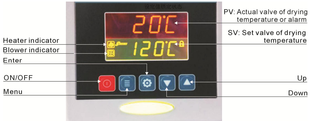
Picture 3-1: Control Panel
