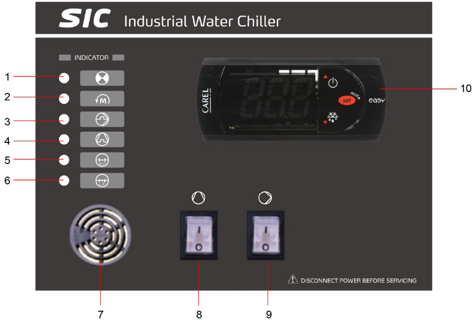
Picture 4-1: Control Panel
