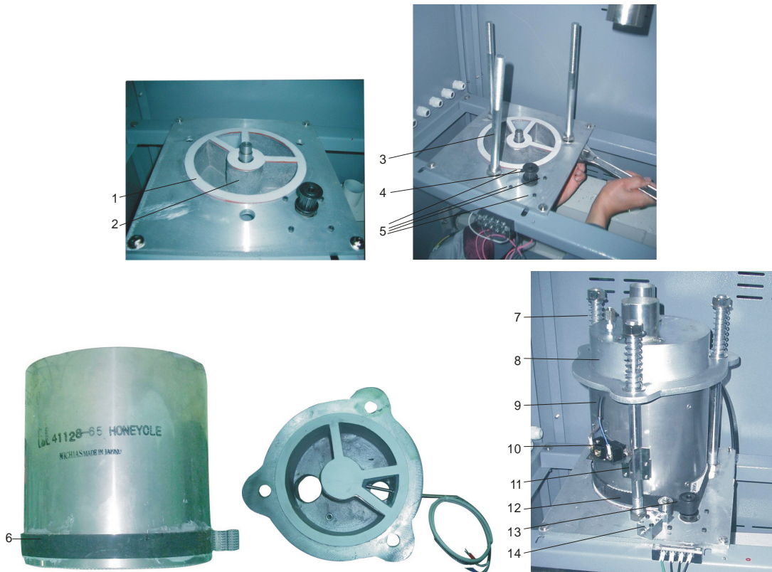
Picture 6-3: Installation of The Rotor
