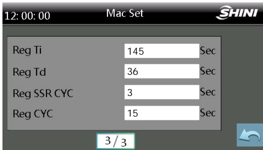
Pic. 4-18: Project Setting-PID Setting Screen
