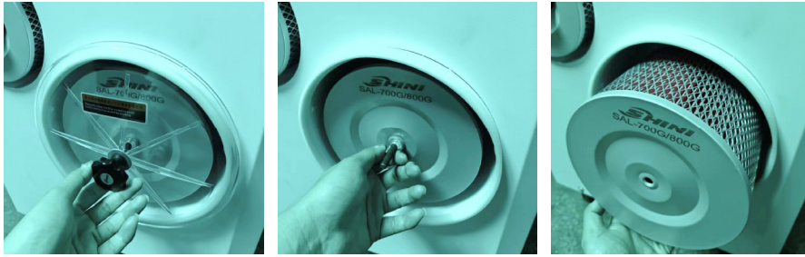
Picture 6-2: Filter Cleaning
