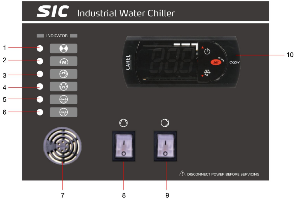
Picture 4-1: Control Panel
