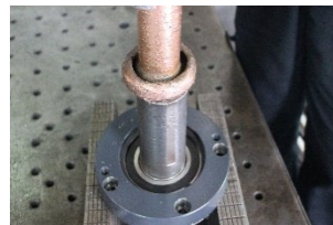
Picture 6-17: Step 1 of Bearing Dismantlement
