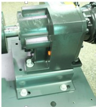
Picture 6-21: Installation of Reduction Gear 2
