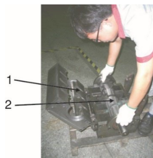
Picture 6-6: Installation of Bearing and Cutter Shaft 2
