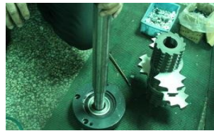
Picture 6-16: Step 3 of Left/ Right Bearing Base Dismantlement
