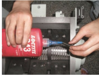
Picture 6-2: Blades Maintenance
