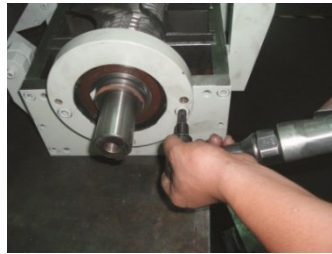
Picture 6-7: Installation of Bearing and Cutter Shaft 3
