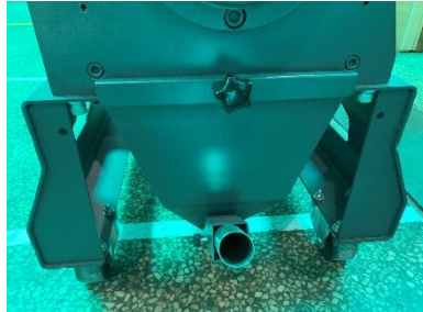
Picture 6-12: Installation of Feed Box, Feed Port and Storage Box 4
