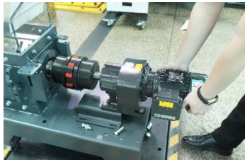
Picture 6-13: Step 1 of Gear box Dismantlement
