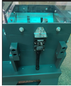
Picture 2-3: Safety Switch
