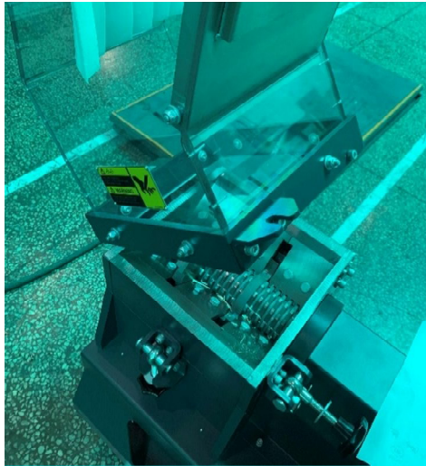
Picture 4-1: Open the Feed Box
