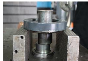
Picture 6-17: Step 1 of Bearing Dismantlement
