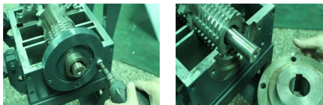
Picture 6-14: Step 1 of Left /Right Bearing Base Dismantlement
