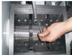
Picture 6-3: Remove the Fixed Blades
