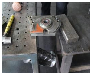
Picture 6-35: Step 3 to Take Out the Blade-rest Shaft
