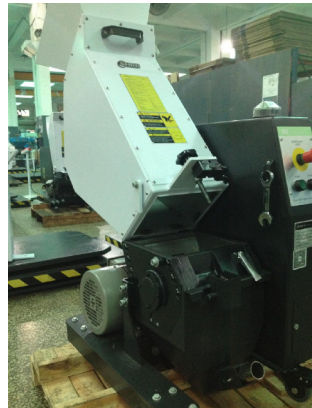
Picture 4-4: Open the Feed Box 2
