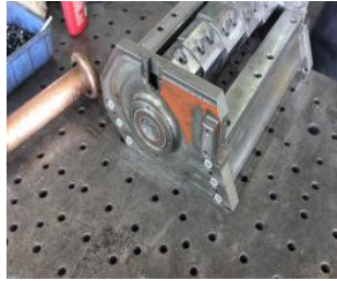
Picture 6-29: Step 1 of Cutting Chamber Dismantlement
