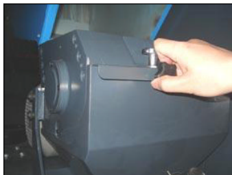
Picture 6-28:Installation of Material Collection Box 4
