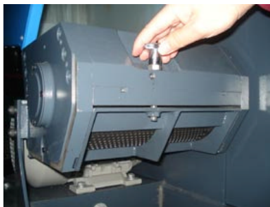
Picture 4-6: Open the Screen and Screen Frame 1
