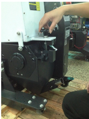
Picture 4-4: Open the Feed Box 2
