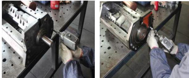
Picture 6-30: Step 2 of Cutting Chamber Dismantlement
