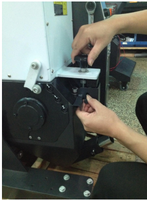
Picture 4-3: Open the Feed Box 1
