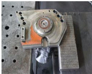
Picture 6-33: Step 1 to Take Out the Blade-rest Shaft
