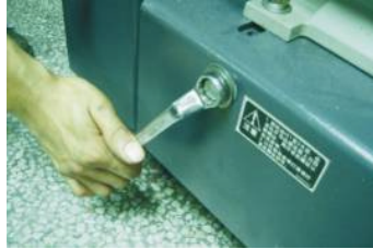
Picture 6-4: Adjustments of V Belts 2
