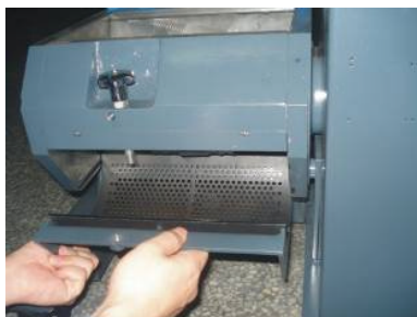
Picture 4-7: Open the Screen and Screen Frame 2
