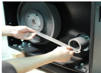
Picture 6-17: Installation of Belt and Belt Pulley 7
