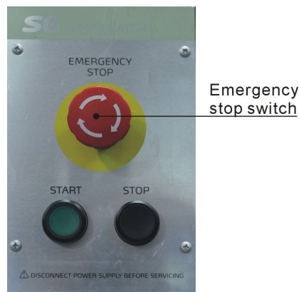
Picture 2-2: Emergency Stop Switch
