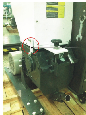
Picture 4-3: Open the Feed Box 1
