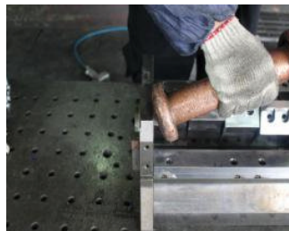
Picture 6-31: Step 3 of Cutting Chamber Dismantlement
