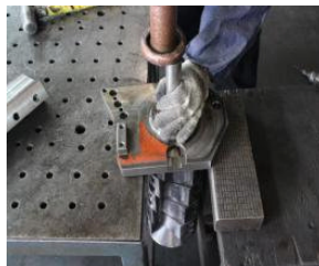
Picture 6-34: Step 2 to Take Out the Blade-rest Shaft
