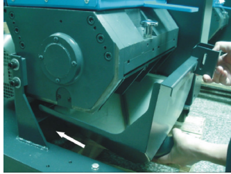
Picture 6-25:Installation of Material Collection Box 1
