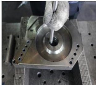
Picture 6-37: Step 2 to Take Out the Bearing
