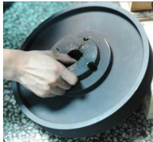
Picture 6-12: Installation of Belt and Belt Pulley 2
