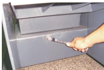
Picture 6-3: Adjust the V-belt 1
