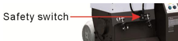
Picture 2-3: Safety Switch
