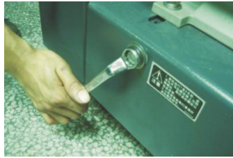
Picture 6-4: Adjust the V-belt 2
