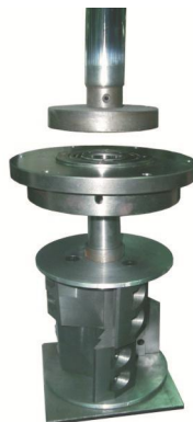
Picture 3-5: Installation of Bearing Block and Bearing
