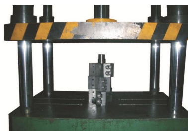
Picture 3-3: Installation of Blade Rest Shaft
