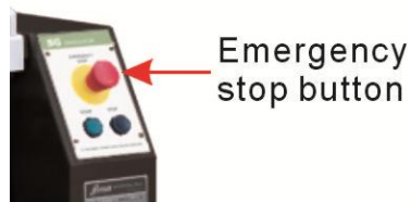
Picture 2-2: Emergency stop
