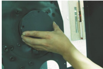
Picture 3-6: Installation of Bearing Cover
