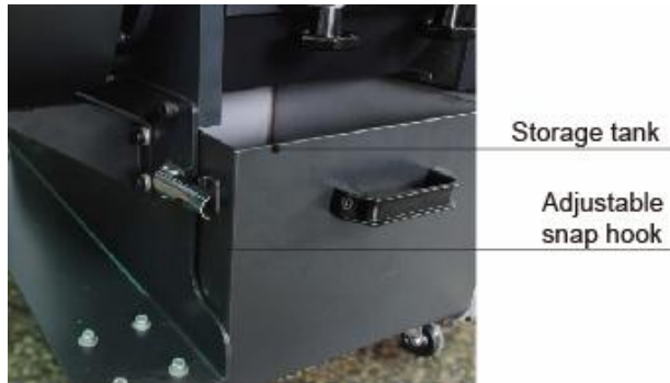
Picture 6-9: Collection Box Installation
