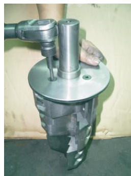
Picture 6-2: Material Fender Installation
