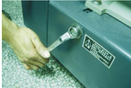
Picture 6-18: Adjustments of V Belts 2
