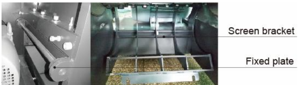
Picture 6-7: Installation of Screen Bracket
