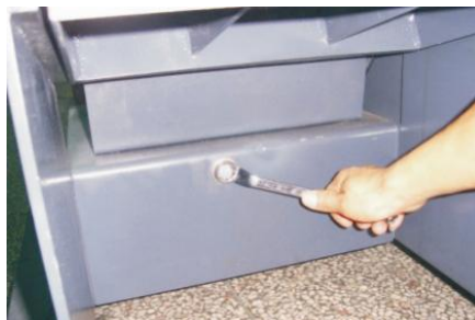
Picture 6-17: Adjustments of V Belts 1
