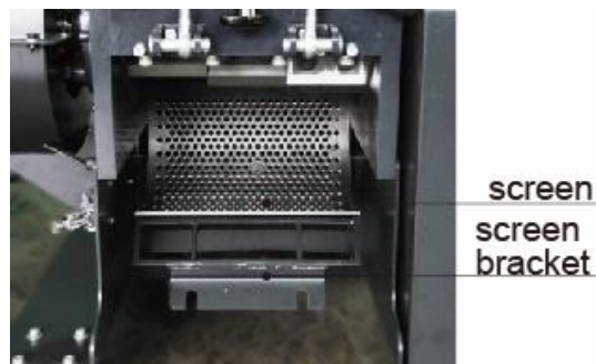
Picture 6-8: Screen Installation
