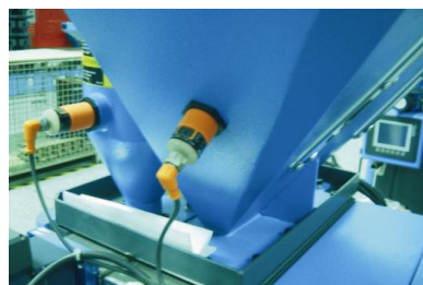
Picture 4-30: Level Switch on Hopper
