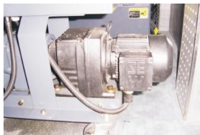
Picture 3-6: Installation of Gear Motor and Coupling
