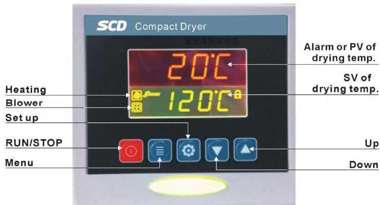
Picture 4-15: Control panel
