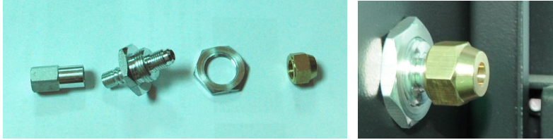
Picture 2-14: Copper joint assembly of original machine
