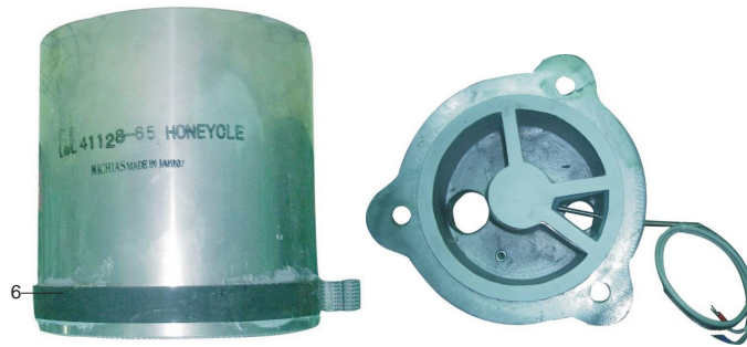
Picture 6-4: Honeycomb-rotor installation steps 3
