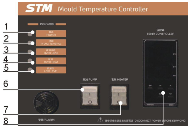
Picture 4-1: Control panel
