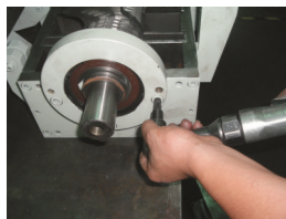
Picture 6-11: Installation of Bearing and Blade Rest 1 3
