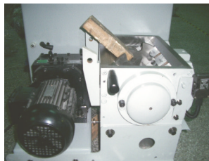
Picture 6-2: Dismantle Fixed Blades
