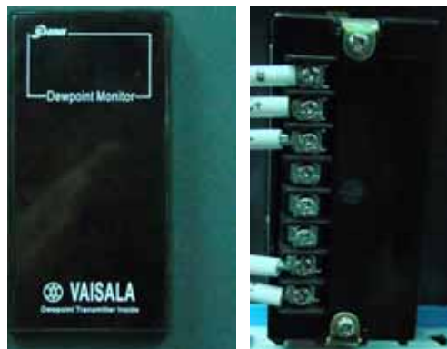
Picture 4-16 : Installation for Dew-point Monitor
