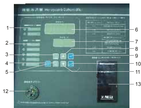
Picture 4-1 : Control Panel
