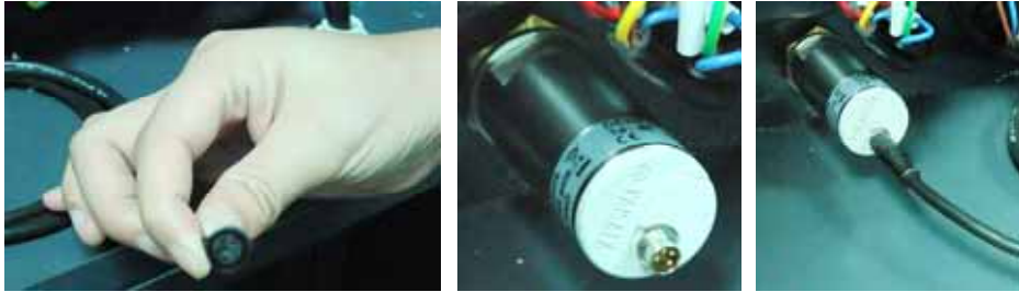
Picture 4-15 : Connection of Signal Wire
