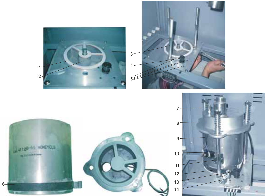
Picture 3-3 : Installation of the Rotor
