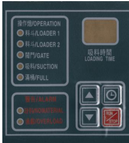
Picture 4-1: Control Panel
