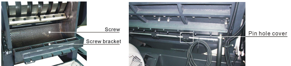
Picture 6-10: Installation of Storage Box, Screen and Screen Bracket 2
