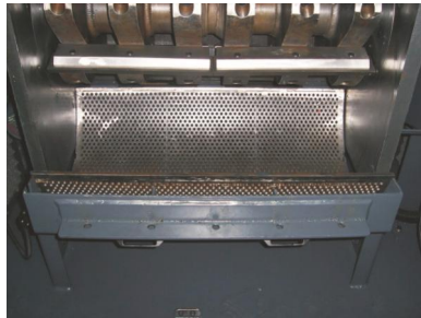
Picture 4-1: Close the Screen Bracket; the Regrind Storage Bin and the Feeding Hopper
