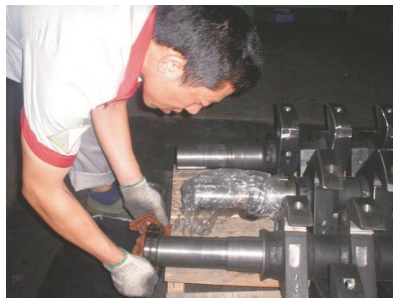
Picture 6-5: Installation of Bearing and Blade Rest
