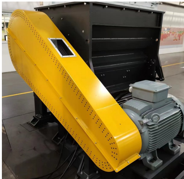
Picture 6-8: Installation of Belt Pulley and Motor 3
