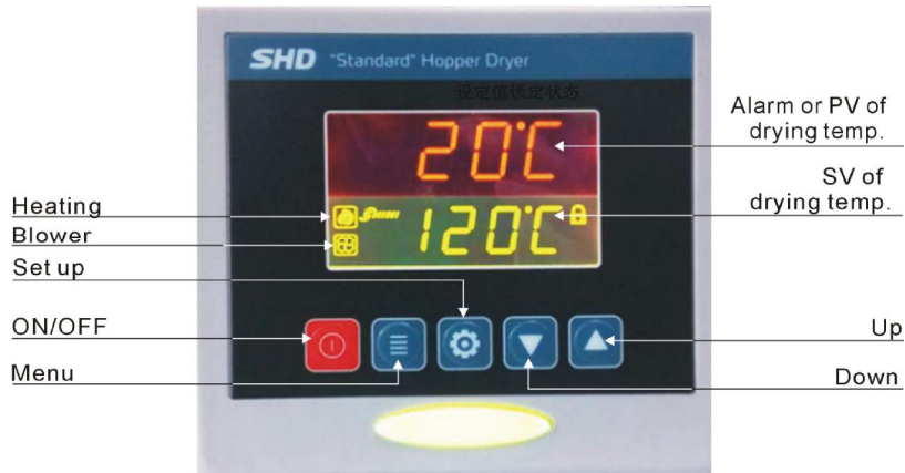
Picture 4-1: Control Panel
