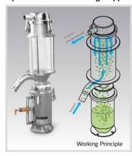
Optical SCD-OP series together with powder- removing hopper which can help avoid stain in the production; material contact surfaces are all mirror polished and collocates conveying system with closed loop to avoid contamination and moisture regain; system has standard configuration high efficiency particulate absorbing filter, which can filter tiny ion of 0.3µm with filter ratio of 99.995%. (Only applicable to SCD-20U/30H-SCD-120U/80H)
