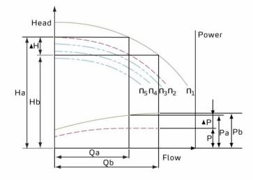
The relation between rotational speed and pump flow, lift and power
