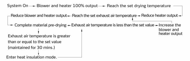
Note: The drying temperature will be decreased in the heat insulation mode.
