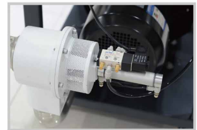
Vacuum breaking valve
