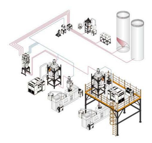
Based on its technology strength and experience in auxiliary equipment field, Shini can meet various kinds of demands from plastics conveying, dehumidifying and drying; mould heating and cooling; regrinds recycling to color management. Adopt intelligent energy-saving control technology to monitor the material processing, Shini can provide different solutions according to different requirements from the customers.
