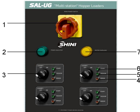
Picture 4-1: Control Panel
