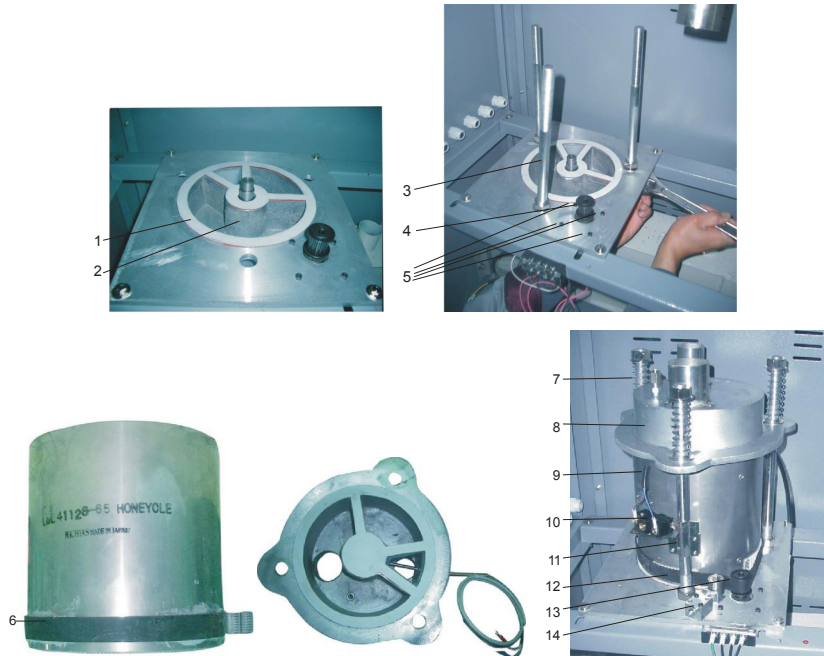
Picture 6-7: Rotor Installation Diagram
